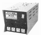
**Power Play.** Electronic Specialists has expanded its computer and office machine AC Power Regulator-Conditioner line. With the addition of the company's 150-watt and 1,500watt units, regulator-conditioner selection can be more closely sized to actual equipment requirements. Features include heavy load start-up capabilities, seven-stage input spike supression, wide-band filtering, sine wave output, and ultraquiet operation for total protection. Contact: 800-225-4876.
