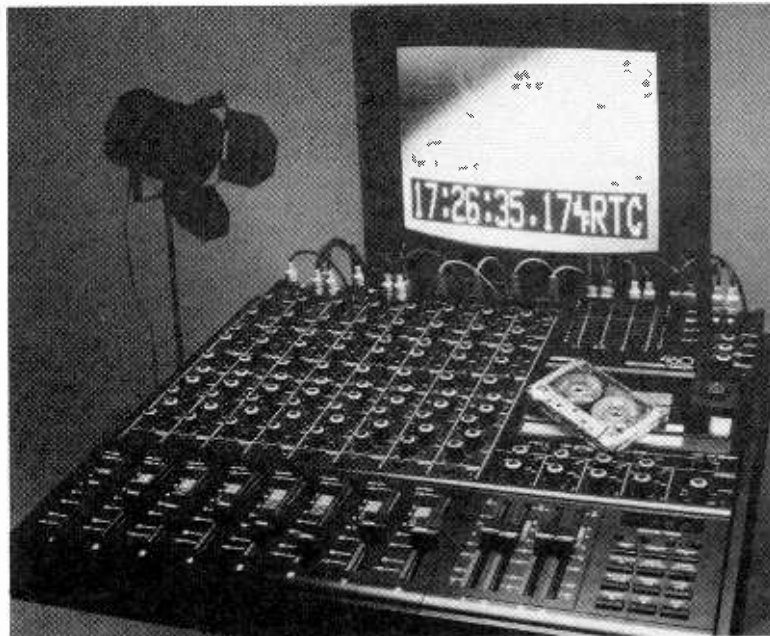
Sync Me Up. This new Fostex 460 Multitracker is the first multitrack cassette/mixer combo to feature SMPTE sync capability for interfacing with video or audiotape recorders.
