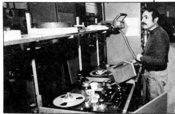
Michel Papaleukas, director equipment maintenance, checks frequency response on a 64:1 duplicating line.
