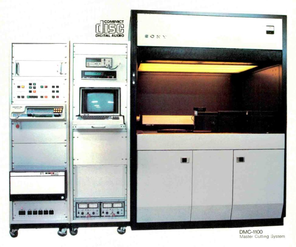
Digital cutting is an exacting step in the process of producing the master digital disc. So, of course Sony has pioneered the development of the complex computer-controlled system that automatically transfers the master digital tape program into the CD master. The Sony DMC-1100 Master Cutting System, along with the CDP-5000 CD Player, and CDA-5000 CD Analyzer work together to provide a flawless result.
