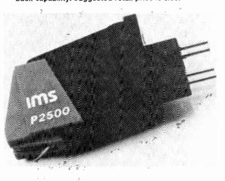
The P2500 from the Nagatronics Corp. in Freeport, N.Y. is one of two new P-Mount induced magnet phono cartridges. It features a diamond elliptical stylus in a low mass cantilever with a non-aging high energy samarium cobalt magnetic activator.
