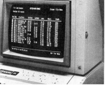
Apple Computer's new monochrome 12-inch video display monitor displays 24 80-character lines with high resolution graphics in P31 green phospher. The monitor also has a tilt mechanism. The U.S. suggested retail price is \$229 and includes a 90-day warranty.
