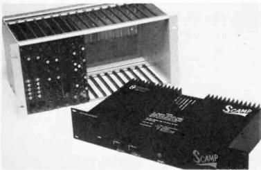
SCAMP SYSTEM—This Scamp card modular signal processing system will be among products shown by Audio & Design Recording Ltd., at the upcoming AES show. The unit embodies the card-module concept within a standard rack-mount frame. It provides a range of signal processing equipment in a space saving, high density format.
