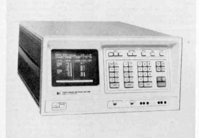
SIMPLE ANALYSIS—Hewlett-Packard of Palo Alto, Calif. offers the new HP3779C/D, a primary multiplex analyzer (PMA) with analog-digital and digital-analog measure for product testing.
