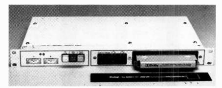
Figure 3. Professional Dolby C encoder module. The C-type NR module plugs directly into the Dolby encoder unit now installed in most duplicating facilities.
