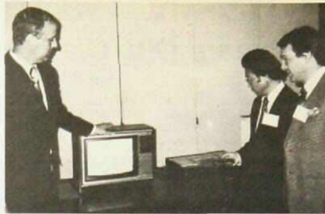
NEW PORTABLE —At right, RCA's Dave Daly holds Hitachi-built portable VHS deck with one-hour charge built-in battery pack; companion tuner/timer, AC power supply charger at left.
