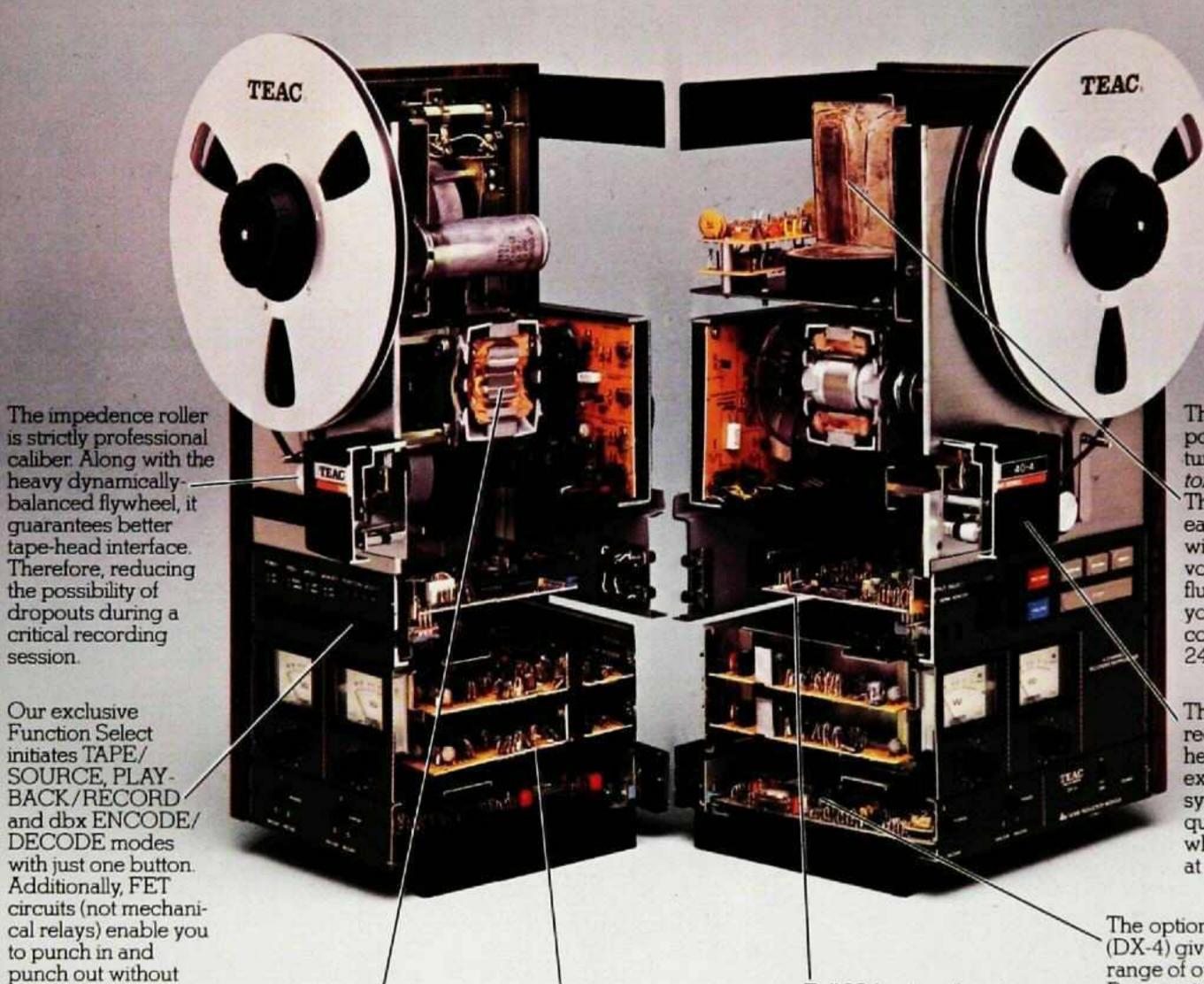
The heavy-duty power supply features a pro-quality toroidal transformer. This assures that each deck function will receive its correct voltages without any fluctuations. Even if your 40-4 runs constantly for 24 hours a day.
