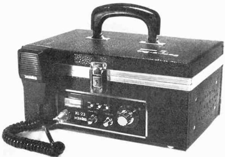
KRIS Tag-a-Long portable AM CB radio is mounted in leatherette travel case with two speakers, built-in antenna, lighter power-plug.
