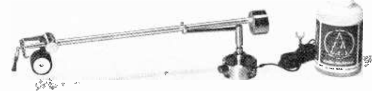
AUDIO-TECHNICA AT6002 disk cleaner has conductive brush, arm to neutralize static build-up, drum reservoir for controlled fluid application.
