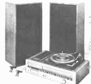
LLOYD'S R973-014 stereo system has AM/FM/MPX receiver, 8-track player/recorder, BSR automatic changer, 2-way speaker systems, new look.
