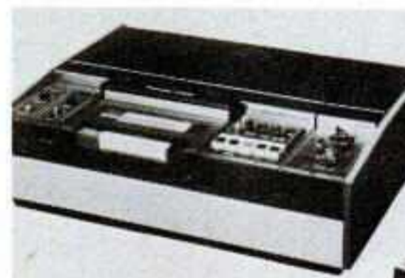
PANASONIC introduces its NV-2125 ¾ inch video cassette recorder with built-in UHF/VHF tuners. Other features are a built-in RF adaptor for playback through a TV, automatic tape threading and drop-out/noise compensator.
