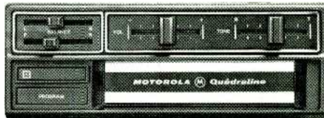
Model TM912S. Under dash mounting. Sliding volume control. Sliding tone control. Separate front/back, left/right balance controls. Cartridge activated on/off switch. Speakers optional extra. 24 transistors. 13 diodes.
