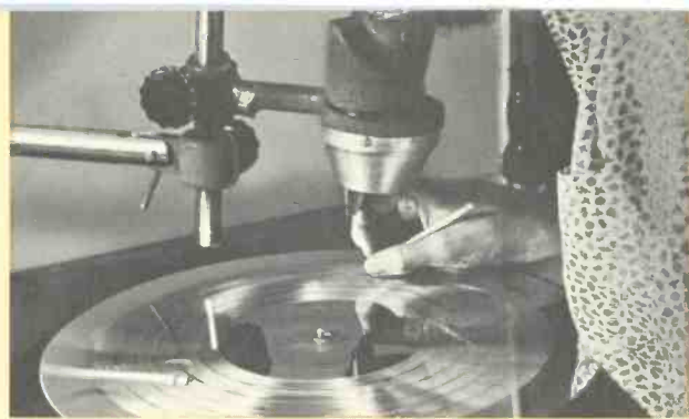
Skilled engravers with years of experience are employed in the preparation of a metal matrix.
