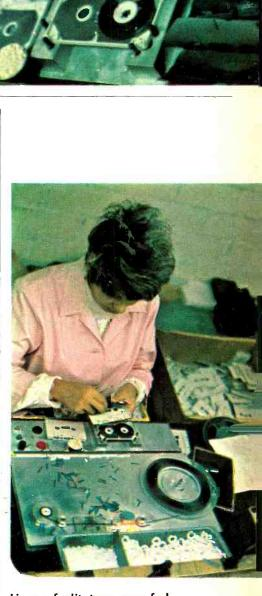
Lines of slit tape are fed onto spools (lef#) before moving to the loading and assemblying process (above) where girls feed the tape into plastic cases.
