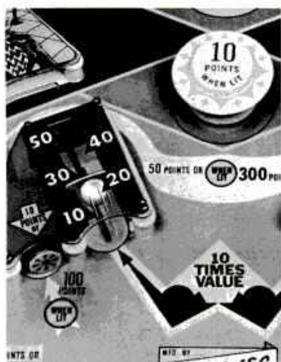
CLOSE-UP view of Vari-Target on D. Gottlieb's new games. There are two targets. When the 10-times-value light is illuminated the ball driven to the scale area indicated by 50 will score 500 points.
