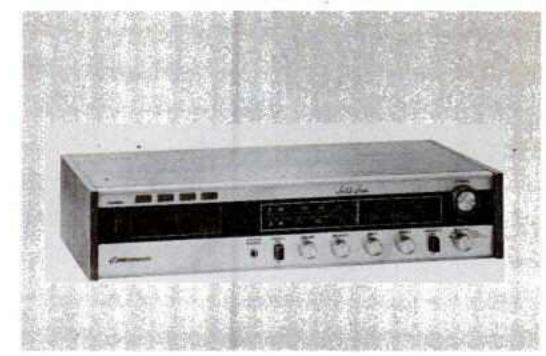
AUTOMATIC RADIO features this home CARtridge entertainment center. Designed as an 8-track player, Model HMX-4000 also plays 4-track cartridges with its Gidget adapter and receives AM and FM multiplex broadcasts.
