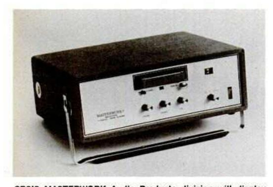
CBS'S MASTERWORK Audio Products division will display its new 4-track tape CARtridge player, Model 4400, which operates on AC, flashlight batteries, a cigaret lighter or can be connected to a boat's battery.
