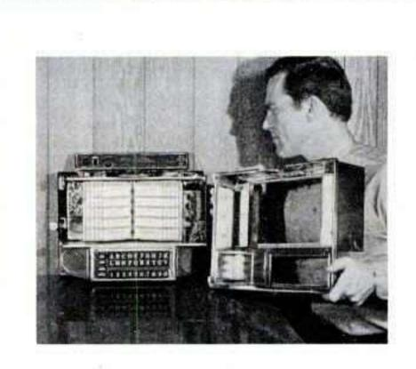
Many exclusive features make service a breeze. When used on counter, the Wall-Ette can be serviced from back without disturbing customers.
