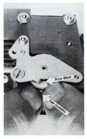
FINGER TIP PRICE CONVERSION is accomplished with the new "Five-Price" select price changer from Coin Acceptors, Inc. Easily reached price wheel cam allows settings for 5, 10, 15, 20 and 25 cents, and is interchangeable with any other Coinco unit.
