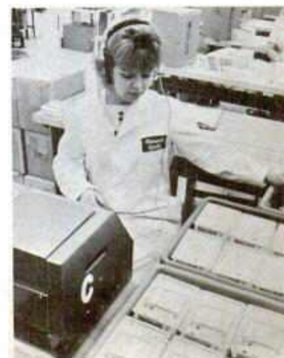
RCA QUALITY CONTROL worker gives finished Stereo 8 cartridges their final audio test before they are shipped out.
