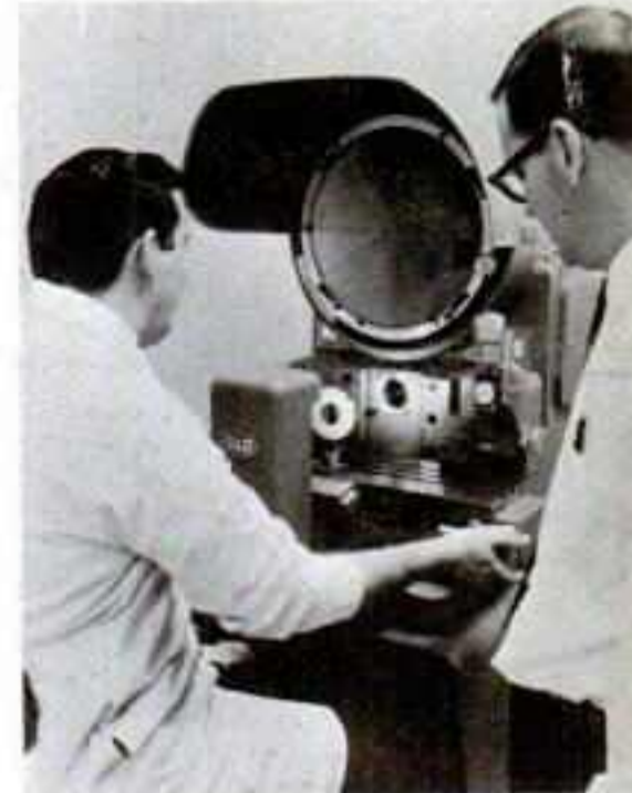
ENGINEERS SCAN AN optical comparator to guarantee the absence of crosstalk on Stereo 8 cartridges. After recording, the track location—revealed by Magna Vista—is measured on this comparator to determine that each track is within tolerance, thus avoiding crosstalk between the channels.
