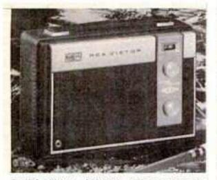
Solid-state eight-transistor Globe Trotter AM portable radio. RF tuned stage, four-inch speaker, peep-hole tuning, earphone jack. Operates on four C batteries. Black textured case. Retails for \$27.50.
