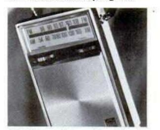
AM/FM pocket radio. Vernier tuning, ferrite rod AM and telescoping monopole FM antennas, eight transistors, has "penguin feet" earphone and nine-volt battery. Wrist strap, two-tone plastic case. Retail price \$19.95.
