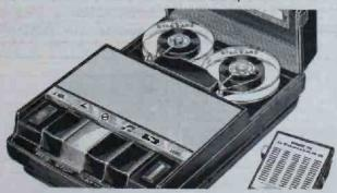
STANDARD FIVE-TRANSISTOR tape recorder. Plays 50 minutes at 1% l.p.s. on 2-inch reel. Four push-button controls, remote control microphone, telephone pick-up, carrying case, six AA batteries. Price \$44.95.
