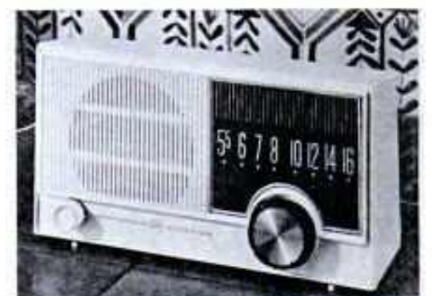
Solid-state AM radio by Motorola. Four transistors, two diode chassis. Four-inch speaker and loudness control. Slimline styling, polystyrene cabinet. List price $22.95.
