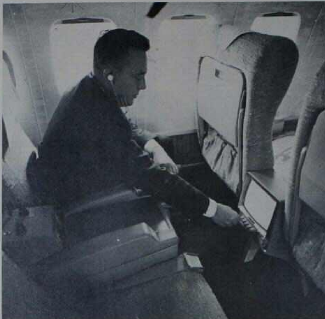
ENTERTAINMENT IN THE AIR. Passenger aboard an American Airlines Astrojet adjusts picture on personal movie screen located between seats in front. This feature is part of a unique entertainment system—giving passengers a choice of movies or stereophonic music—being installed on American's fleet of 707 and 720 Astrojets.
