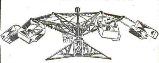
The Frolic is a fast, thrilling ride that appeals to all ages. Requires a 60-ft. space, loads easily on one 32-ft. semi-trailer, has a capacity of 16 adults. Ride can be supplied with a gas engine for partable operation or electric motor for permanent locations. This is a full-sized ride built at a price that the professional operator can afford to pay.
