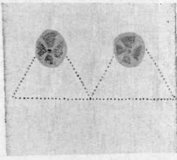
Stereo speaker enclosures must have wide angle dispersion horns to spread the sound of each channel over as broad an area as possible.
