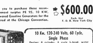
Engine: 4 cylinder, 4 cycle L-head, water cooled, rated 35 horscpower at 1800 RPM. Generator: 120 or 240 volts, single phase 60 cycle AC; rated power 10 kw. at power factor of 1.0; 12.5 k.v.a. at 80 @ power factor. (Voltage change is accomplished by changing jumper connection on terminal strip.)
