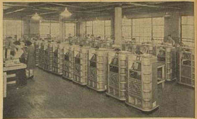
A PART OF THE ASSEMBLY LINE at O. D. Jennings & Company, Chicago, on telephone music equipment. Here is the final assembly cabinet department where finishing touches are made before the equipment goes on to the inspection department.
