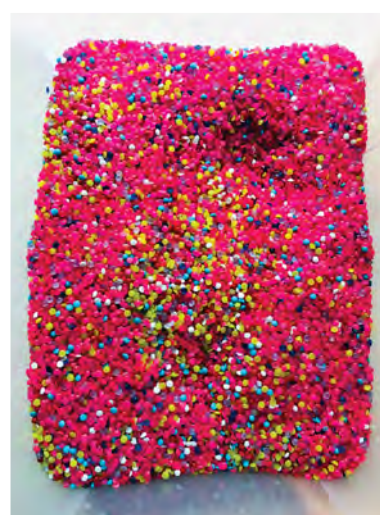
Above: A Deepgrooves staff member with the Phenix Alpha pressing machine, which processes around 100 records per hour. Left: Deepgrooves' calcium zinc pellet blend.
