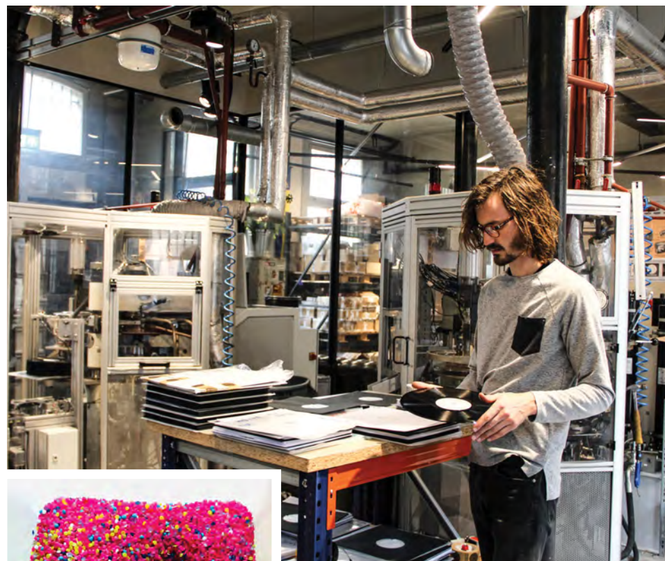
Above: A Deepgrooves staff member with the Phenix Alpha pressing machine, which processes around 100 records per hour. Left: Deepgrooves' calcium zinc pellet blend.
