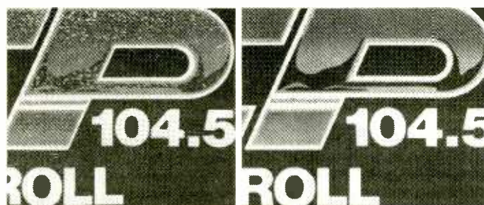
After the test, the equivalent of a year in the weather, note the peeling, fading and cracking in the "label" type product (left). The Communication Graphics decal (right) still looks great.
