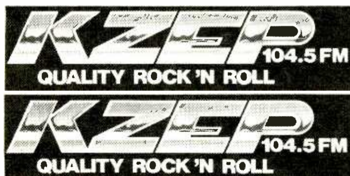
In a General Motors developed test, stickers are aged the equivalent of one year's exposure to the elements. The top sticker was produced by Communication Graphics, the bottom by another company. As you can see, they appear identical "off-the-press."
