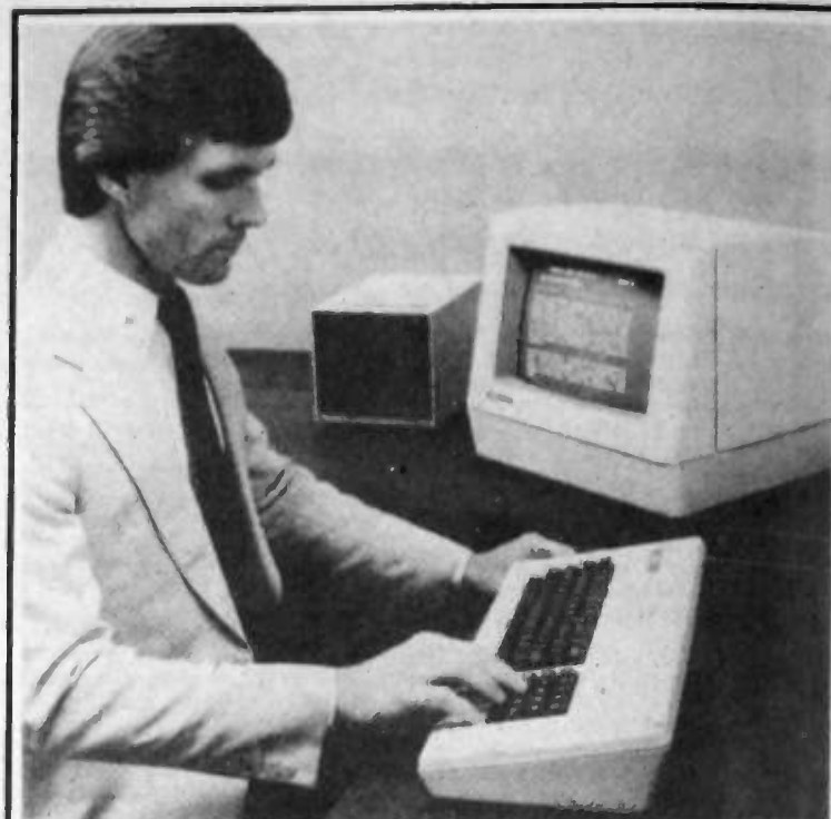
The Xerox "820" in action. Seen from left are the disc drive storage unit, the CRT, and the touch-type keyboard.
