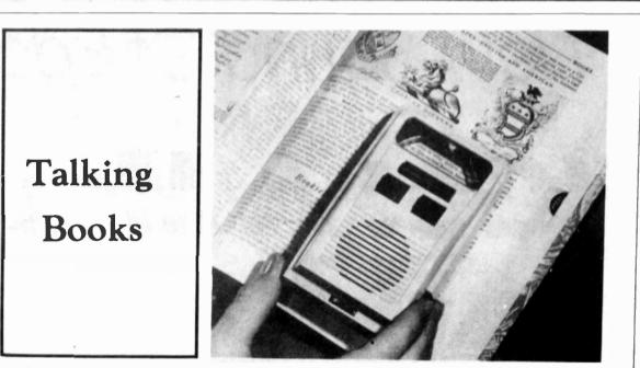
The Microsonics Corporation has recently introduced a compact audio/visual system capable of bringing sound to the printed page. The system utilizes a handheld microphonograph that plays a transparent audio disc mounted on printed material to provide up to 90 seconds of audio information.
