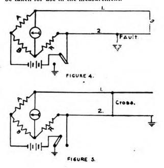
In the first case, that of a ground, proceed as follows: Putting the wire of lowest resistance per mile at the bottom of the bridge, as shown in Figure 4, with the three-point switch to right, A and B being equal, the resistance unplugged in R when balance is obtained, will be the resistance of the loop. Suppose the result to be 630 ohms.
