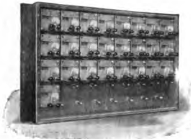
AUTOMATIC CALLING DEVICE FOR TRAIN DESPATCHERS' OFFICE (Cover Removed) SIZE 22 1-4 X 13 3-8 X 3 INCHES
