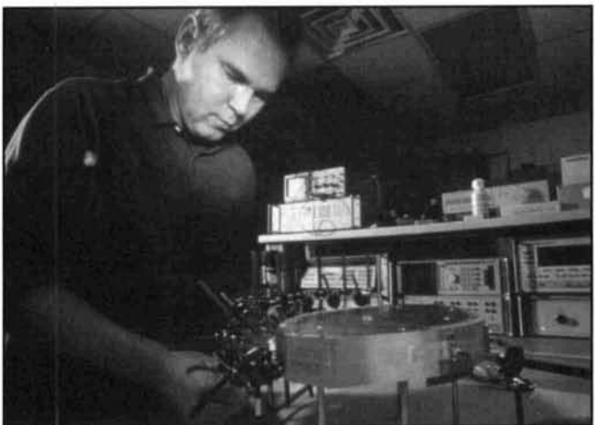
Photo B. Otto Rausch attaches waveguides to test Rotman lens.
