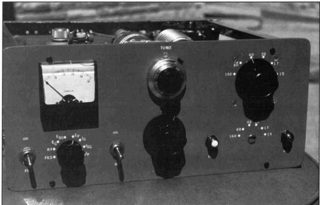
Photo B. The front panel of the W5LAJ linear. Note unused input bandswitch in the lower right-hand corner. See explanation in the text.
