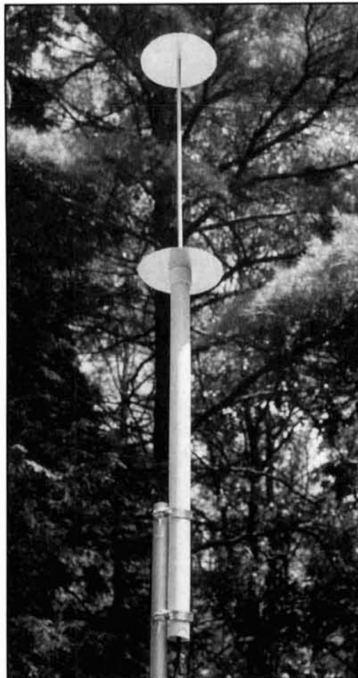
Photo A. Discpole antenna mounted for service on a metal mast. Note that PVC mast isolates antenna from the conductive support pipe.
