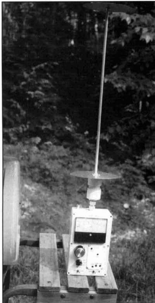
Photo C. Discpole using alternative base assembly. In this configuration, the antenna may be suspended by a nylon line or sill-mounted (like a bird-feeder) using an insulated bracket.
