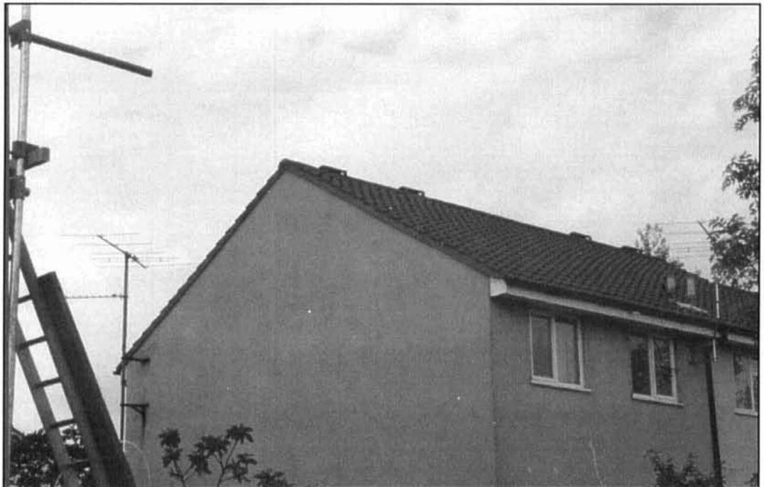
Photo B. The two 110-MHz antennas that form the basis of the interferometer.
