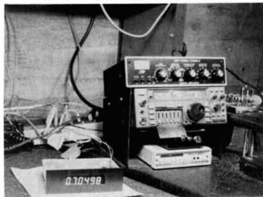
Photo D. Remote display connected to ICOM 735. Case was made from surplus pc board by K7YLM.
