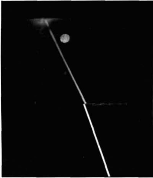
Photo B. Aquarium demonstration. Effect of refraction at a near 90-degree angle of incidence.
