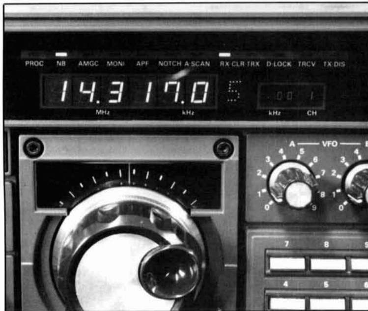
Photo B. The 10-Hz display has been implemented behind the front panel of the FT-ONE.
