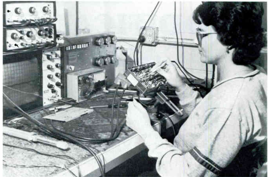
Note "custom test set" to speed up trouble shooting amplifiers
