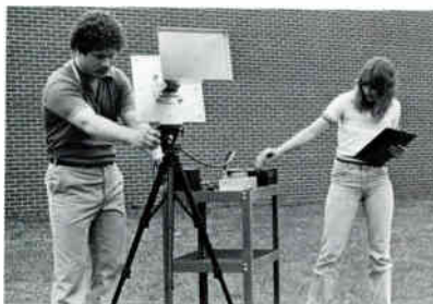
Measuring frequency, azimuth, bearing and polarization of TI with the "do-it-yourself" equipment kit.
