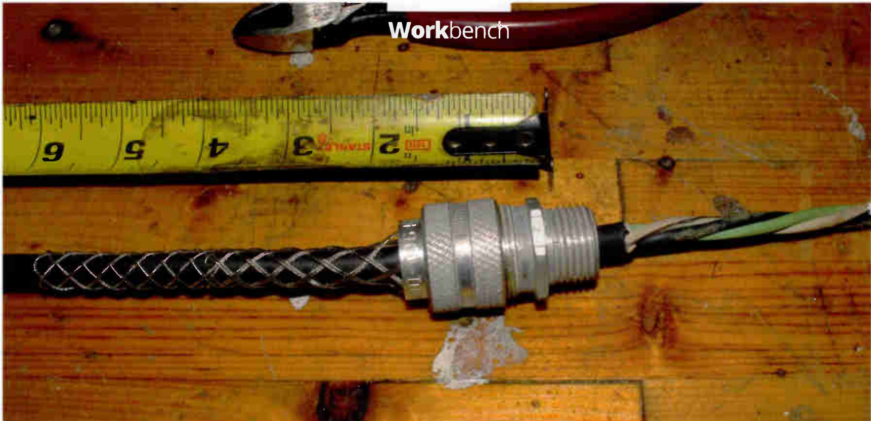
Above Fig. 2: By choosing the appropriate cable connector and strain relief, you guard against future problems.
