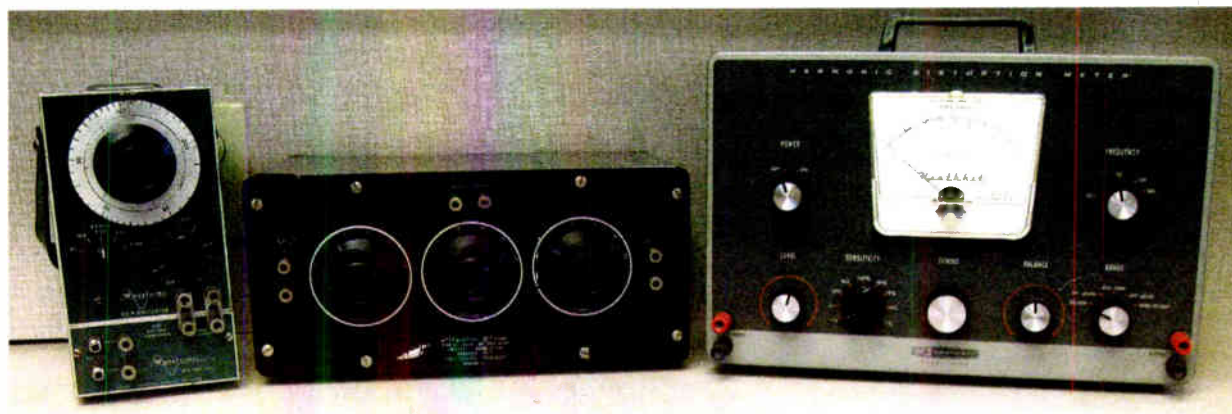
The workbench of a 1970s small- or medium-market station might include a Waveforms 510-B audio oscillator, Daven VT-795-6 attenuation network and Heath IM-12 distortion meter.
