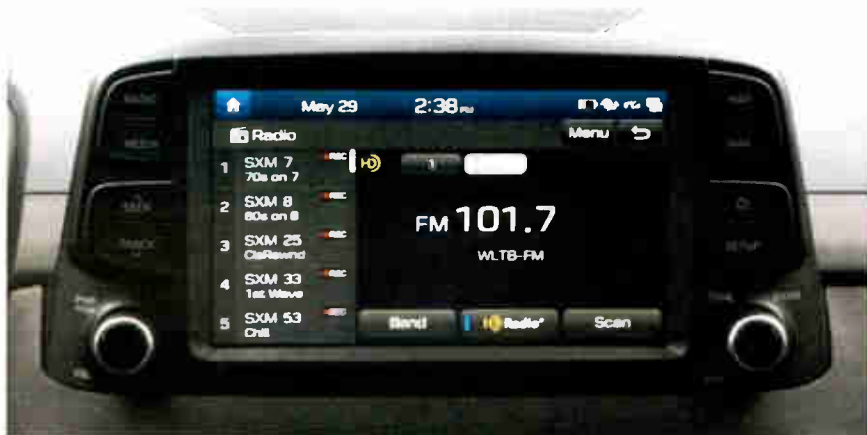
An HD2 signal being broadcast. Note the mix of knobs, touchscreen and buttons for control.
