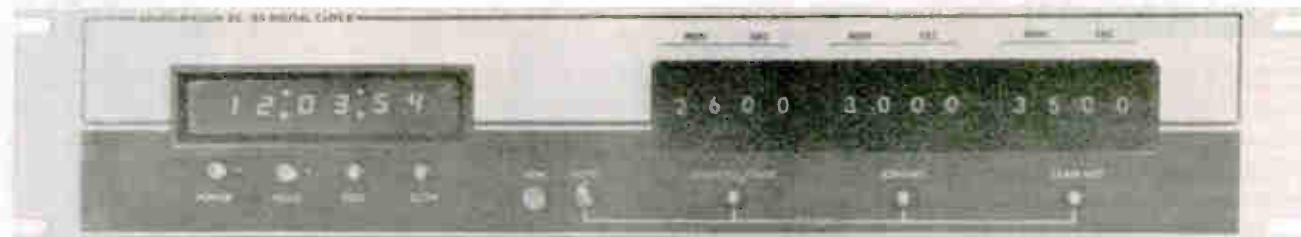
Master clock and network join functions were performed by the Sparta DC-24.
