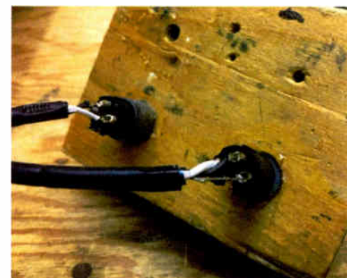
Fig. 5: Freshly-soldered connectors using the “third hand”
