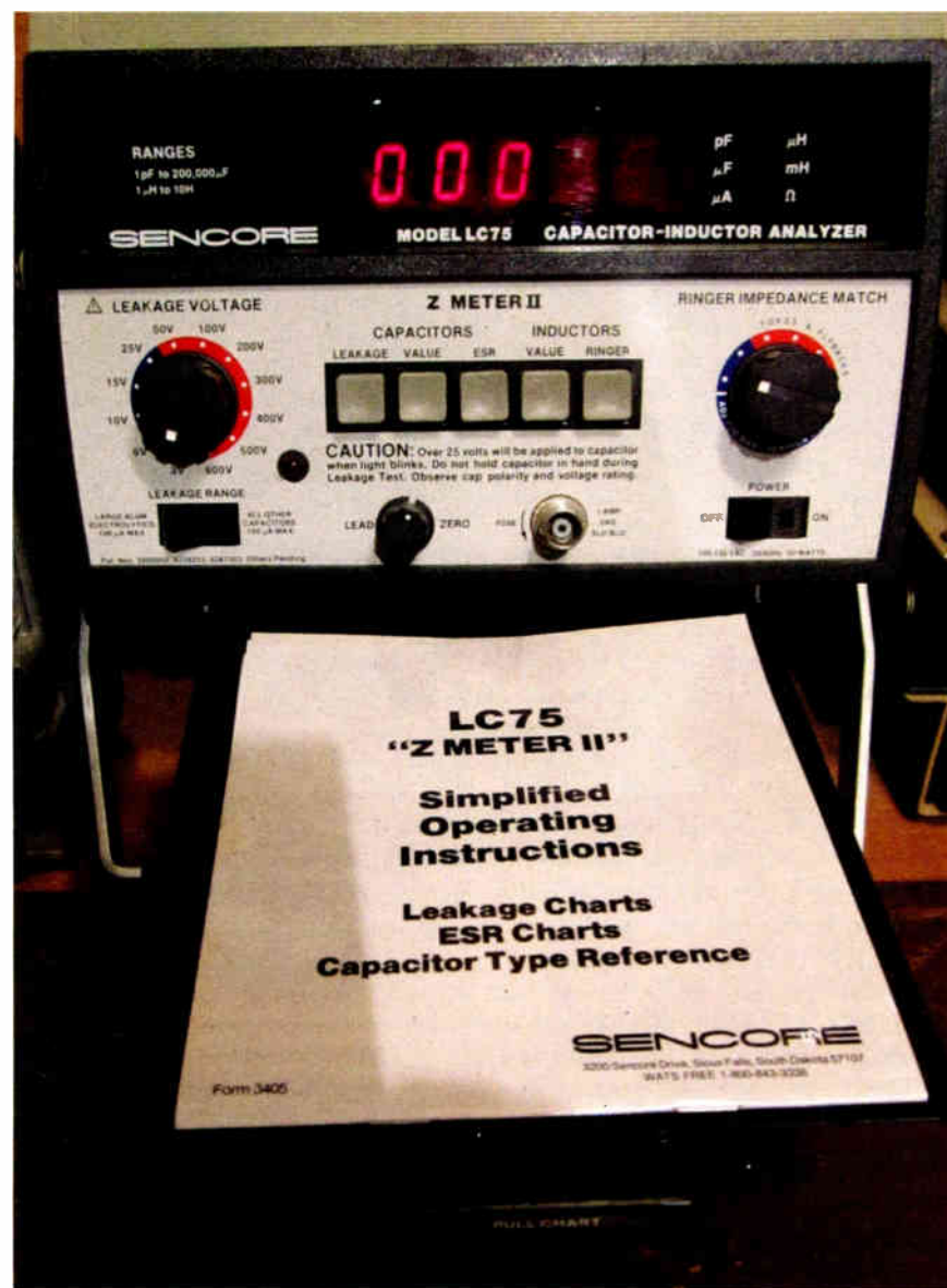
Fig. 1: The Sencore LC75 can be used to test for high equivalent series resistance.
