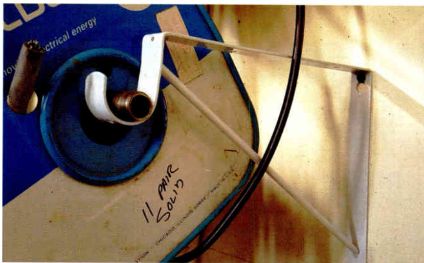
Fig. 1: An end cap screwed on the end of the support pipe would prevent the spindle from slipping off its support.
