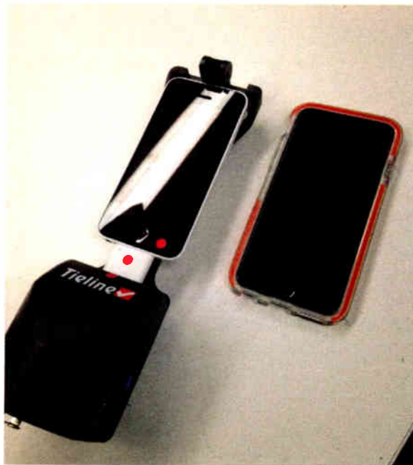
Fig. 1: Tieline's Mic Adapter for the iPhone 4. Notice that the larger phone won't fit.
