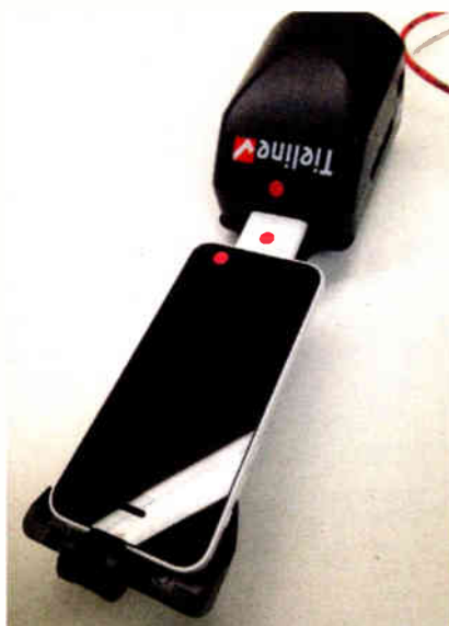
Fig. 5: The completed Mic Adapter has been modified for the larger iPhone.
