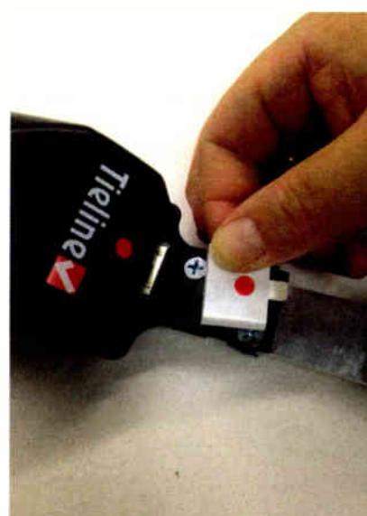
Fig. 6: The headphone jack is marked with a colored dot, and a spring strain relief plug is used.
