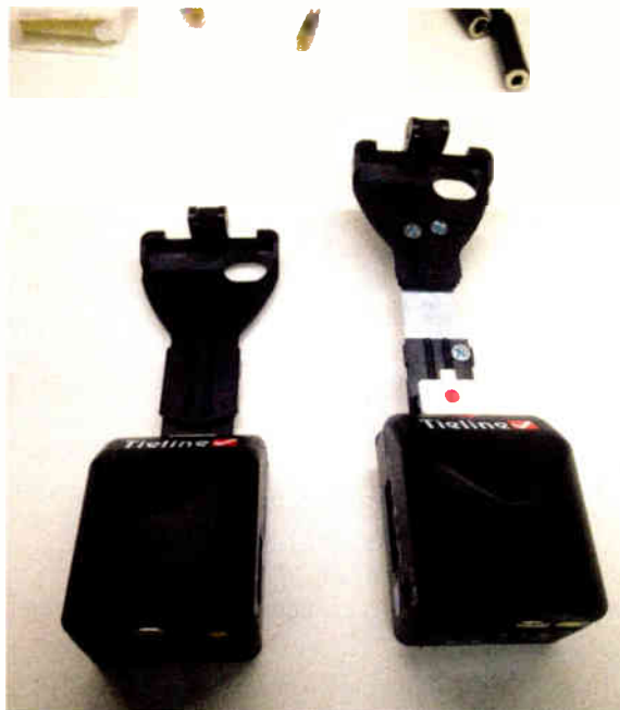
Fig. 2: The Mic Adapter with its metal extension bracket is viewed from above.
