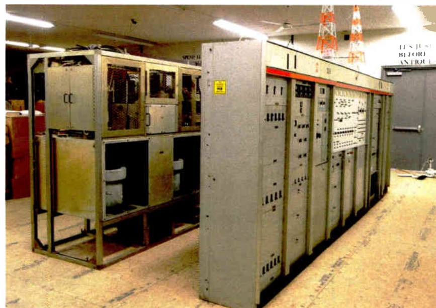
The Collins 821A-1 250,000-watt transmitter is shown after its reassembly at the AWA Museum in Bloomfield.
