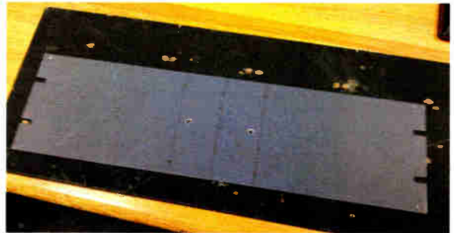
Fig. 2: Center the panel to the monitor and mark the four mounting holes ...
